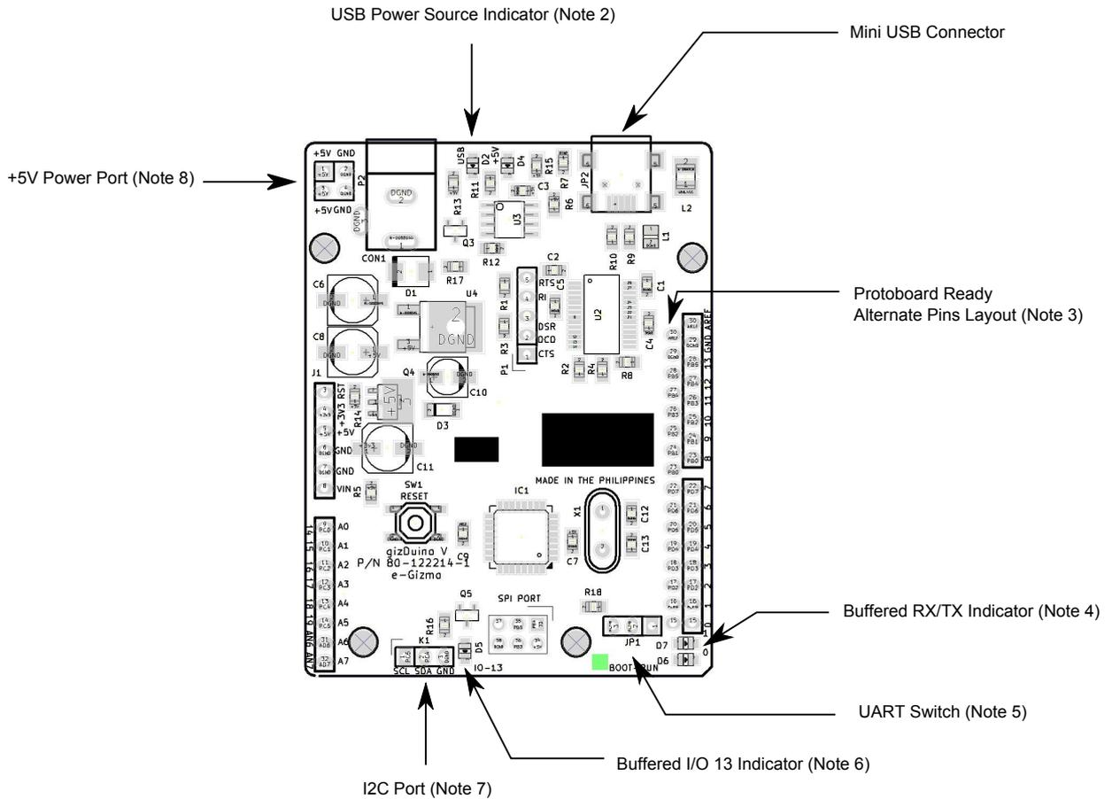
**gizduino5** is the latest iteration of our continually evolving Arduino compatible series of programmable controllers. It provides added features suggested by users including:
