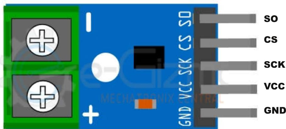
**Figure 1: Major parts of MAX6675 Thermocouple Temperature sensor module.**
