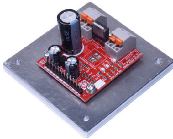
Figure 3. The Little Hulkster mounted on a aluminum heatsink. This 72.5 square x 6mm thick aluminum heatsink enables the driver to drive even bigger motor that requires more amps.
