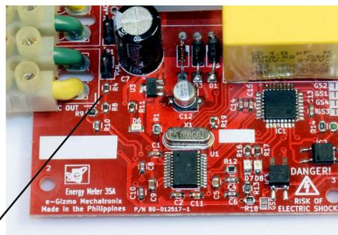
Offset calibration jumper location shown with the jumper already removed.
