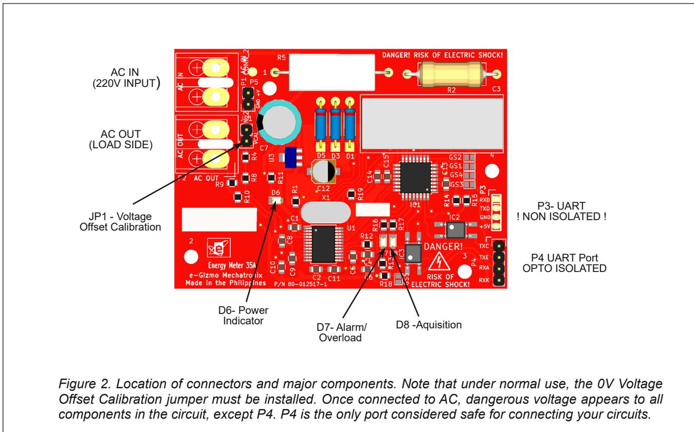
Figure 2. Location of connectors and major components. Note that under normal use, the 0V Voltage Offset Calibration jumper must be installed. Once connected to AC, dangerous voltage appears to all components in the circuit, except P4. P4 is the only port considered safe for connecting your circuits.
