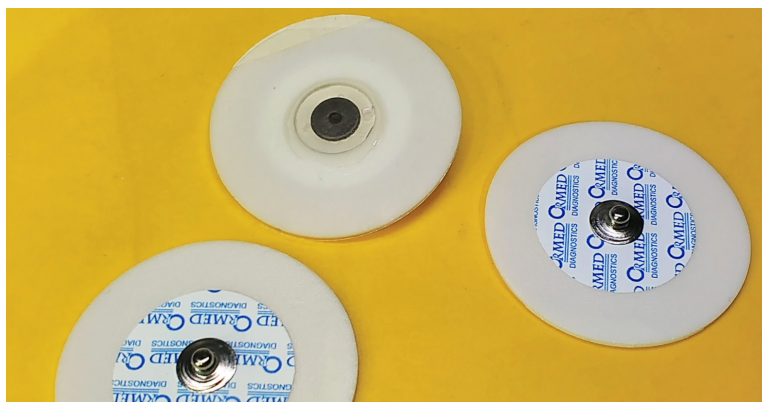
Figure 2. Input noise rejection relies heavily on the quality of electrical contact with your body. This can be achieved only with the use of good electrodes. Cheap disposable electrodes, such as those shown in the photo, will do an ample job when used correctly.
