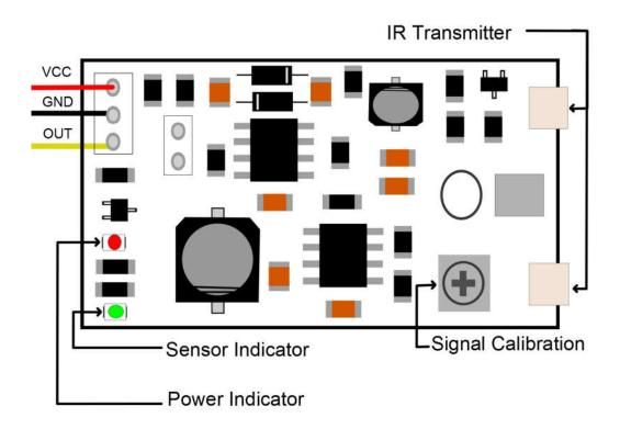
Figure 1. Compact Proximity Collision sensor & its major Components.
