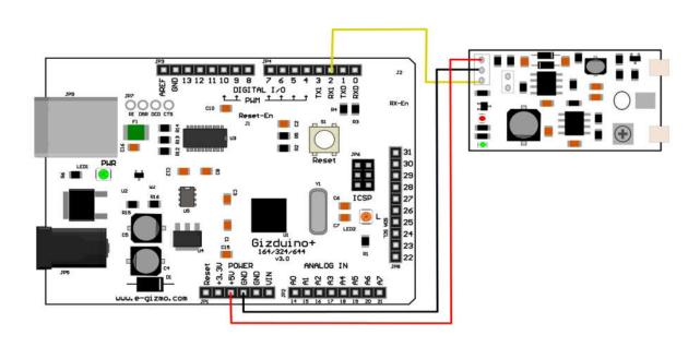
**Figure 2.** Compact Proximity Collision Sensor Connected to a gizdDuino + w/ ATmega644P microcontroller.
