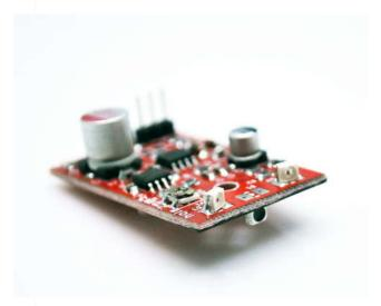
The Infrared Proximity-Collision Sensor detects objects apporximately as far as 72mm(2.8 inches) from the sensor's face. The infrared beam makes it relativley insensitive to ambient light and color (of the target object). Applications include non contact object detection and collision sensor for mobile robots.
