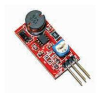
eDC-2420 Step Up DC/DC converter can generate up to 24VDC output from a single +5V input. Available output power ranges from 2.5W with 5.0V input, rising in proportion to the input up to 7.5W at +12V input.
