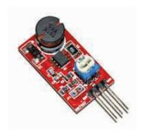
eDC-2416N Negative Output DC/DC converter. From a single +5VDC source, it can generate a negative output voltage of up to -16VDC at 1.6W. It is possible to adjust the output voltage up to about -22VDC, but available output power drops to 0.6W. Increasing the input voltage to +6.0V will make available power climb back to 1.6W. At +12V input, as much as 3.8W is available at -22VDC output.
