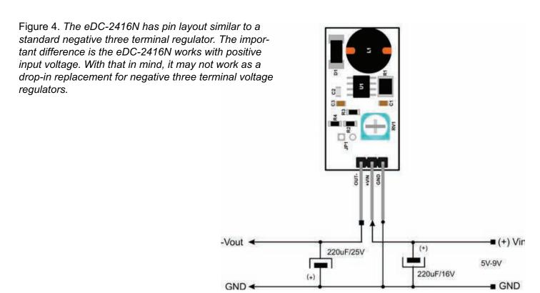
By combining the above circuits, a split +/- output power supply circuit from a single voltage source can be easily constructed.
