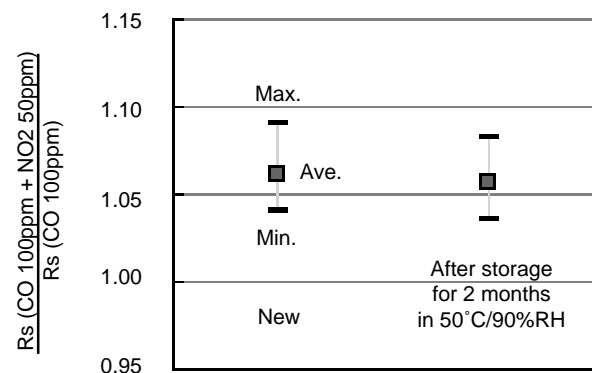
Figure 19 - Effect of high temperature/humidity
