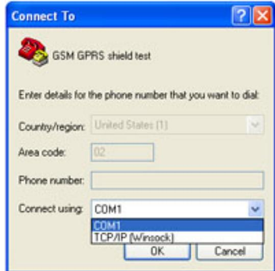
Second, Replace this with the COM port in which the GSM modem is attached to. To know which 'COM' you used, go to ("My Computer">, "Properties">, hardware tab>, "Device Manager">, "Ports">).
