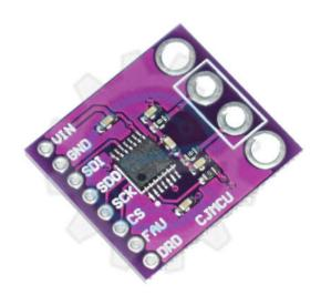
MAX31856 performs cold-junction compensation and digitizes the signal from any type of thermocouple. The output data is formatted in degrees Celsius. This converter resolves temperatures to 0.0078125°C, allows readings as high as +1800°C and as low as -210°C (depending on thermocouple type), and exhibits thermocouple voltage measurement accuracy of ±0.15%. The thermocouple inputs are protected against overvoltage conditions up to ±45V.
