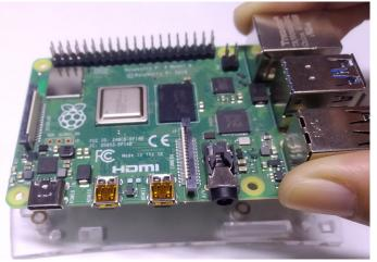
3. Put the 4 screw (2x10mm) on by using a screw driver.
