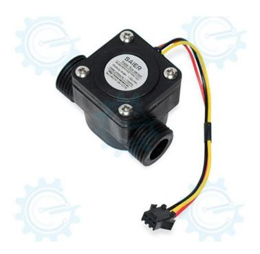
**SEN-HZ21WA Flowmeter** can be used to accurately measure liquid volume and rate of flow flowing through it. It outputs digital pulses at a frequency in proportion to the rate of flow. Accumulated number of pulses, on the other hand, gives an accurate measure of the liquid volume. Compatible in all gizDuino boards and MCUs.
