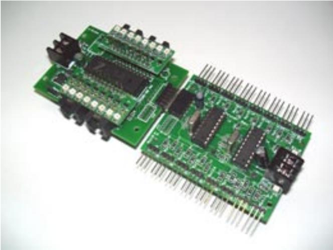
*Figure 5. You can install quickly and just as easily a Servo Driver controller module with the Sequencer board. Simply plug to join them together forming a complete Servo motion controller circuit.*
