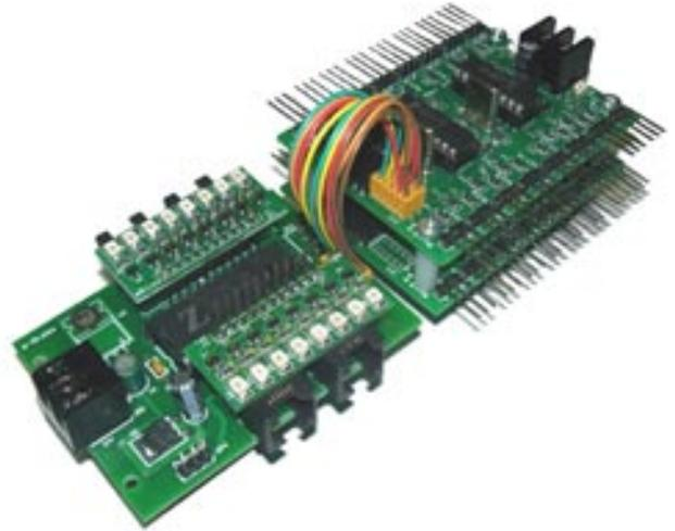
*Figure 7. A Servo Motion Controller configuration with two Servo Driver Controller installed. The lower Servo Driver module connects through JP2, and the upper module connects through the Sequencer JP3. This will allow independent control of up to 32 servo motors.*
