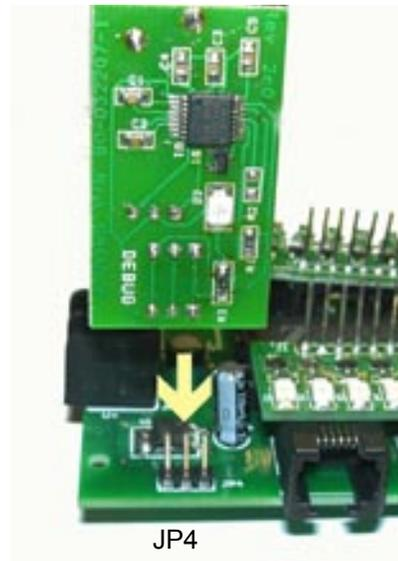
Figure 3. The programming cable is plugged on to the Sequencer board through JP4, with the programmer board component side facing out.
