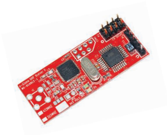
Figure 1. The Multi-Channel Data Transceiver is available in 2 variants – MUDT-433 operates at ISM 433MHz, while MUDT-315 works at ISM 315MHz.
