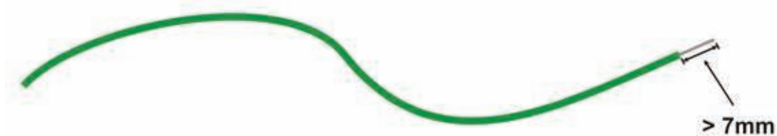
Figure 3. Wire Stripping Guide. The stripped portion should be at least 7mm long.
