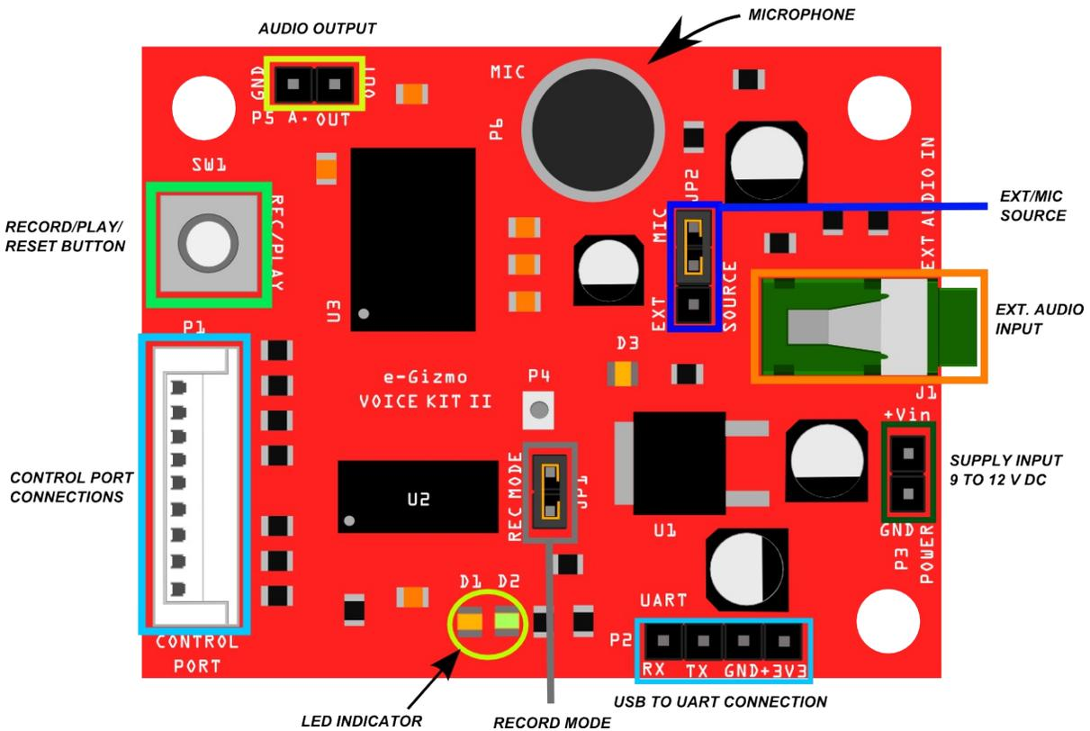
**Figure 1.** VOICE KIT II terminals, connections and LED indicator.
