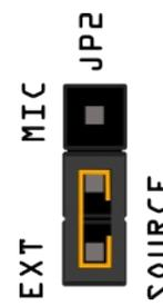
**Figure 4. Jumper settings for using the external audio source**
