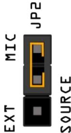
**Figure 3. Jumper settings for using on-board microphone**
