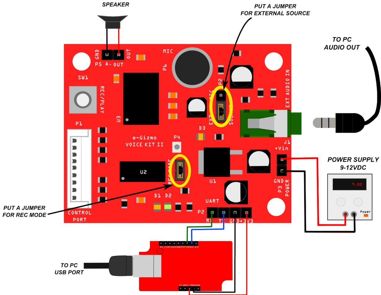
**Figure 7.** Wiring Diagram of Voice Kit II using the External source for sounds recording.
