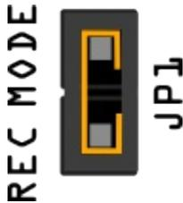
**Figure 5. Jumper settings for enabling chip recording mode**
